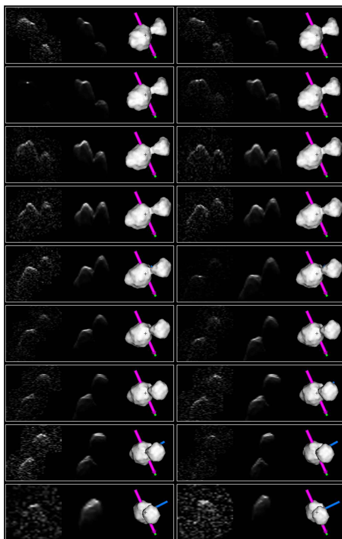
Fig. 2: Fits of the radar-derived shape model of asteroid (68346) 2001 KZ66 to the radar data. Each three-image sub-panel is made of: the observational data (left panel), echo simulated from the best-fit model (middle panel), and plane-of-sky projection of the best-fit model (right panel).
